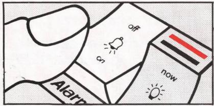
The alarm switch has two positions, OFF and ON.
