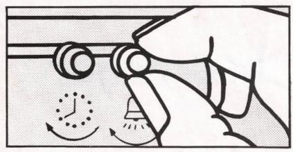
Set the alarm time by turning this knob at the rear clockwise.
