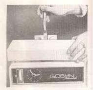
Rotate adjustment knob: Clockwise i.e. direction marked – to reduce loudness, anticlockwise i.e. direction marked + to increase loudness.
